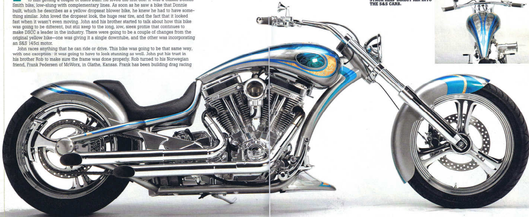
HOLES DRILLED INTO THE FRONT SIDE OF THE VELOCITY STACK HELP DIRECT AIR INTO THE S&S CARB.
