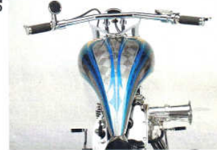
HOLES DRILLED INTO THE FRONT SIDE OF THE VELOCITY STACK HELP DIRECT AIR INTO THE S&S CARB.
