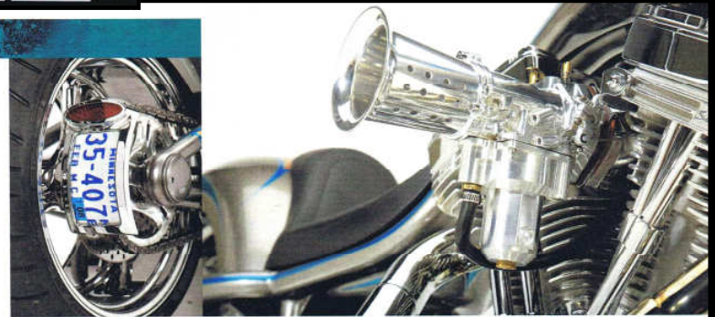
HOLES DRILLED INTO THE FRONT SIDE OF THE VELOCITY STACK HELP DIRECT AIR INTO THE S&S CARB.
