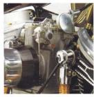
great, swears its maker. "It does away with all that spitting, sputtering and stumbling so common to stacks," Kirk explains. "The screen does a great job of straightening out and evening out the airflow." The piece is timeless and traditional, just like the rest of the bike.
